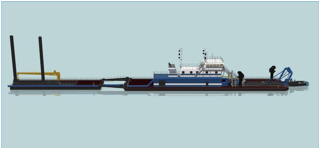
Rendering of custom 24" dual pump Marlin Class dredge
